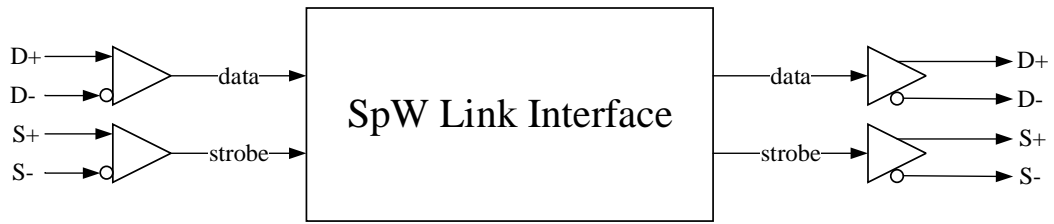
Figure 6.2: SpaceWire LVDS signaling
