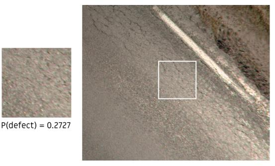
Figure 15. Case of the ResNet101 model predicting a false negative due to lack of context.
