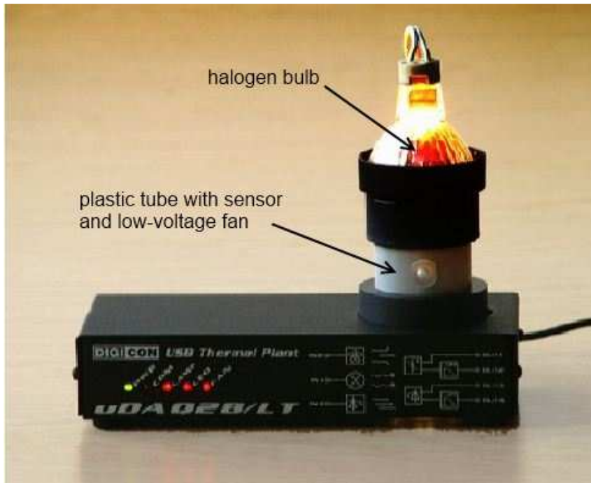
Figure 10. Thermal educational plant from Slovak University of Technology.
