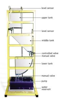
Figure 2.1: Multitank system
